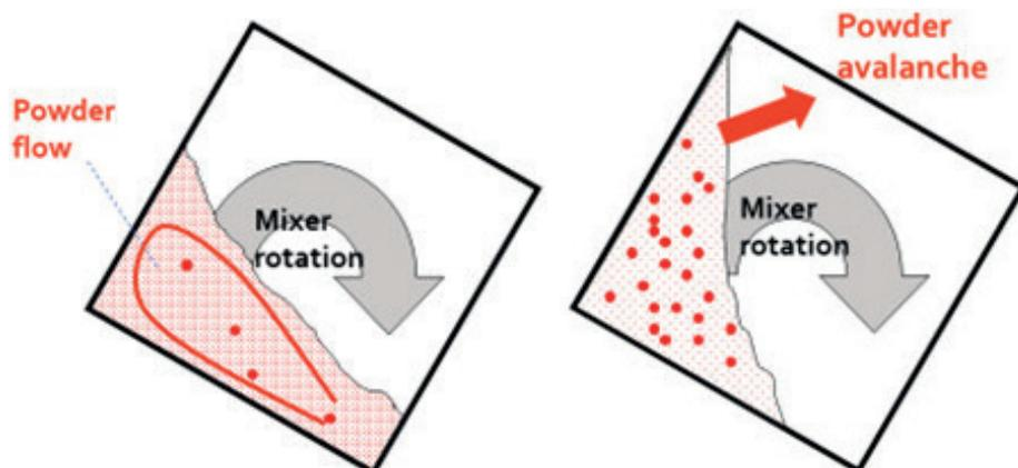
Figure 1: Free-flowing powders tend to set up a rolling motion inside the powder bed, resulting in ball milling of the API agglomerates. Poor-flowing powder tends to avalanche and results in less motion inside the powder bed and less ball milling of API agglomerates.
