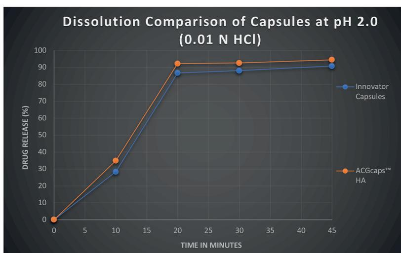
Figure 2: Dissolution profile of ACGcaps™ HA versus innovator capsules containing dabigatran etexilate mesylate pellets. (Apparatus: Modified Basket; Capsule size: 0; Speed: 100 rpm.)
