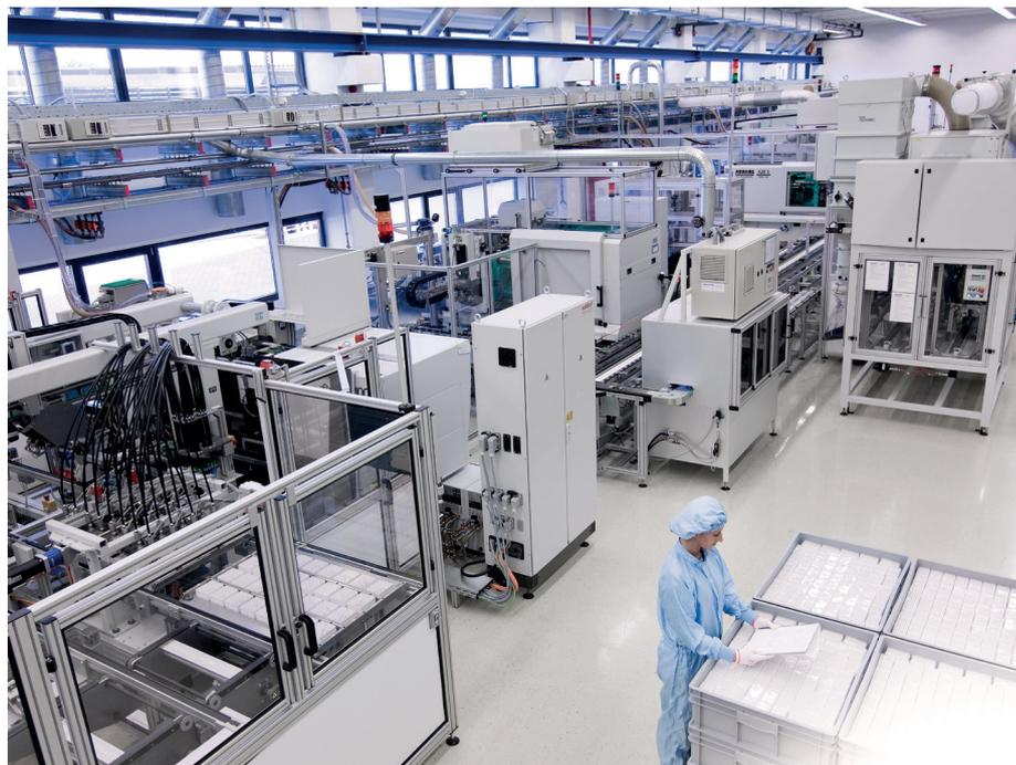
Figure 2: Stevanato Group has more than 160 injection moulding machines at three locations in the US and Germany for GMP, ISO 8 and ISO 7 cleanroom production.
