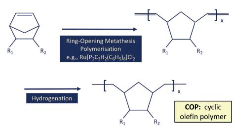
Figure 1: Structure and synthesis of a COP. Poly(norbornene) is represented where R1 and R2 are hydrogen.
