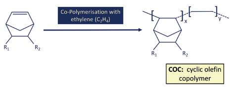
Figure 2: Structure and synthesis of a COP. Poly(norbornene-co-ethene) is represented where R1 and R2 are hydrogen.
