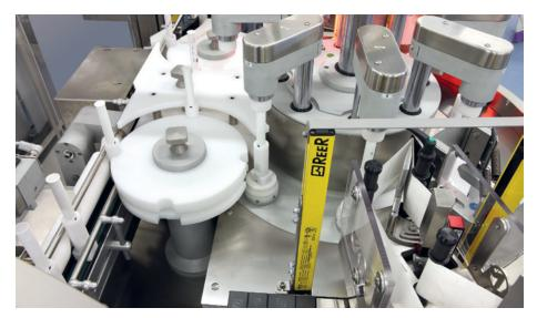
Figure 2: The RE 302 2T twin-head labeller wraps a label around the devices and applies labels on the front and back too.
