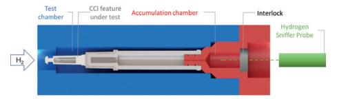
Figure 2: Illustration of a tracer gas CCI fixture. Gas is supplied to the test chamber. If a leak is present, the gas concentration will increase in the accumulation chamber.
