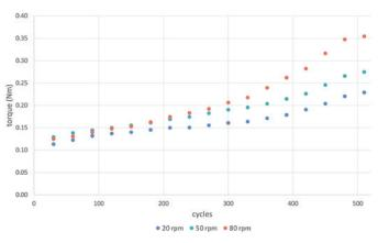
Figure 1: Torque as a function of number of cycles at three different speeds for EVEON's original micropump.
