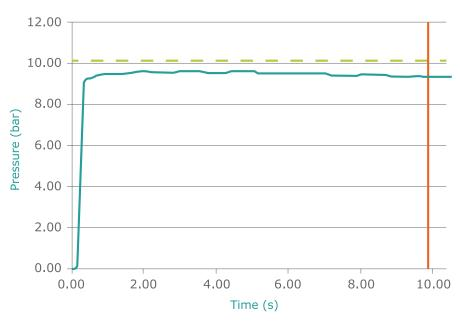
Figure 2: Pressure in a liquefied gas-powered autoinjector during injection.
