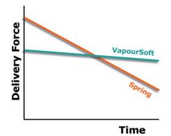
Figure 1: Change in force applied to a syringe in an autoinjector with a standard spring (red) and a liquified gas-powered system such as Bespak's VapourSoft (blue).
