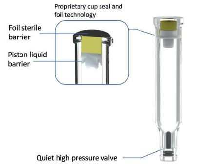
Figure 1: Illustration of seals and CCI interfaces present in Oval's ArQ Bios high viscosity primary drug container (1 mL).
