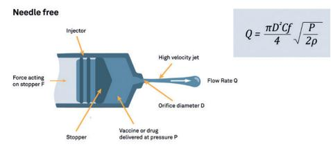
Figure 3: For a needle-free injector, delivery is through an orifice and the flow rate is characterised by the Bernoulli equation.
