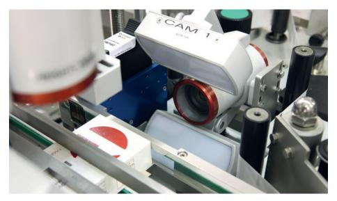
Figure 3: The BL A-420 labeller performs serialisation, stamping and sealing operations.
