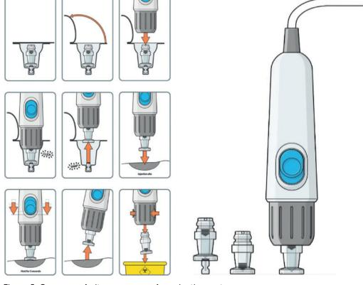
Figure 5: Compressed nitrogen powered vaccination system.
