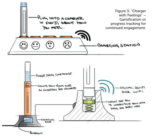
Figure 4: "Weigh the Pen" – Passive or minimal extra use step dose tracking.
