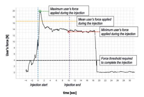
Figure 4: Illustration of a typical user's force-time curve.
