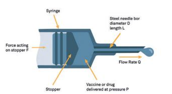
Figure 2: For a conventional hypodermic syringe and needle, flow rate is characterised by the Hagen-Poiseuille equation.
