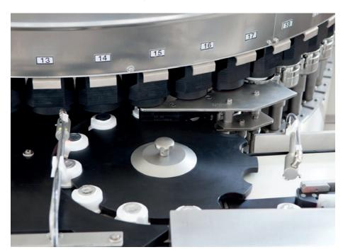
Figure 5: Image of an in-line vacuum decay CCIT method used during production. Photo courtesy of Bonfiglioli Engineering Srl.
