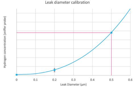
Figure 3: Graph showing a typical calibration curve for hydrogen a sniffer test fixture. Error bars:  $1\sigma$  (n=5).
