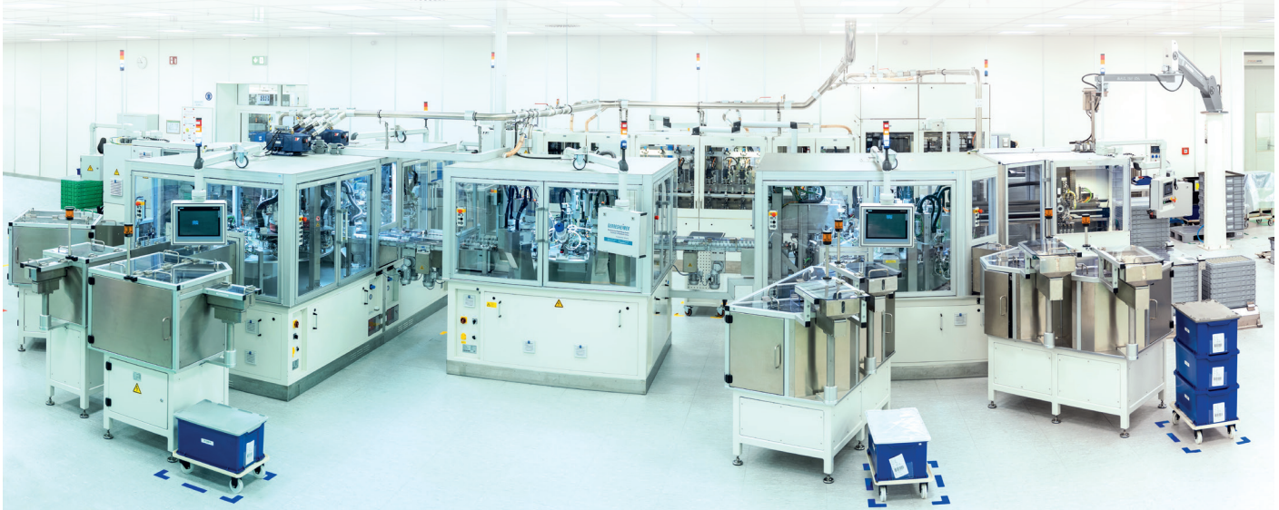
Figure 3: High-volume line for the assembly of the Respimat® reusable inhaler housing module in a clean-room ISO class 8 in Pfreimd, Germany.
