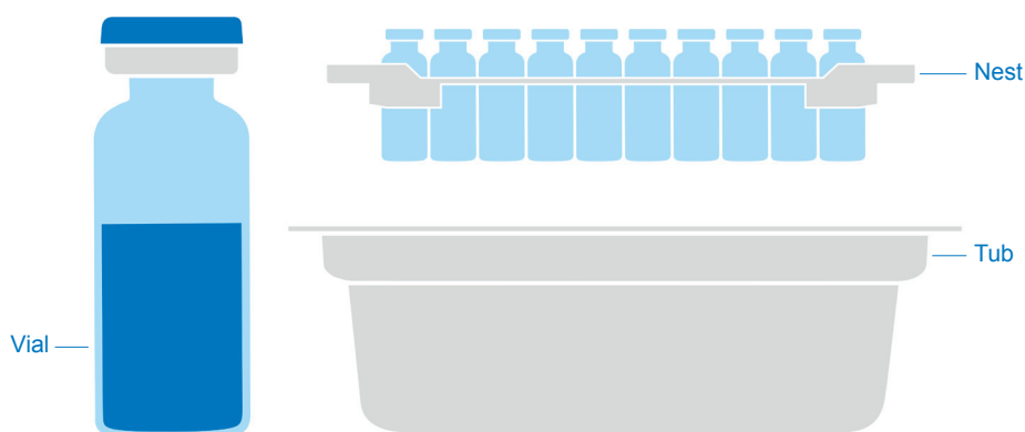
Figure 1: Components of a sterile ready-to-use packaging solution.
