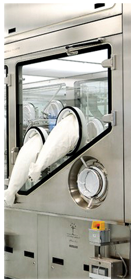
Figure 2: swissfillon’s rapid transfer port used for ophthalmic fill & finish.
