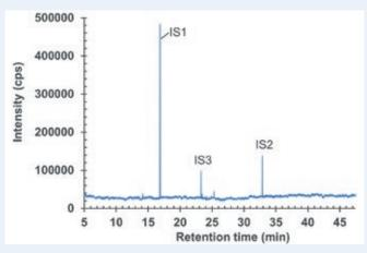
Figure 7: GC-MS chromatogram of polymer syringe barrel after extraction in water (pH 9.5).
