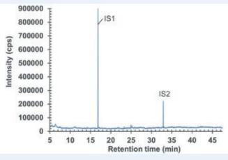
Figure 8: GC-MS Chromatogram of polymer syringe barrel after extraction in IPA/water (1:1).
