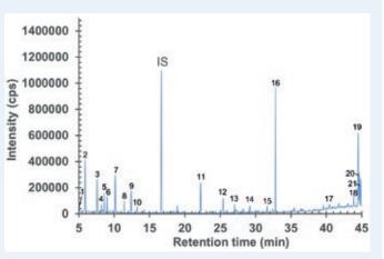
Figure 5: HS-GC-MS chromatogram of rubber stopper component after incubation at 150  $^\circ C$  for 45 minutes.
