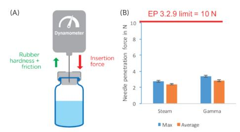
Figure 1: Measurement of needle insertion force. A) Representation of the experimental setup. B) Representation of the maximum insertion force and average insertion force measured for steam- and gamma-sterilised PremiumCoat<sup>®</sup> 20 mm stoppers. The data were collected after two years of ageing and using 21G 3-bevel needles.
