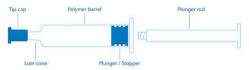
Figure 2: Polymer syringe system.
