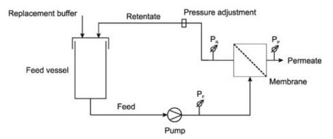
Figure 1: Representation of diafiltration setting.<sup>2</sup> (Source: WikipediaDorian).
