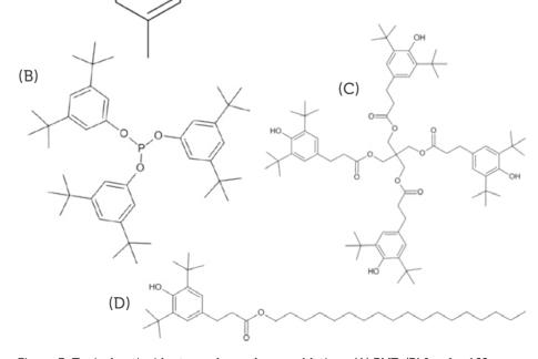
Figure 3: Typical antioxidants used as polymer addatives. (A) BHT, (B) Irgafos 168, (C) Irganox 1010 and (D) Irganox 1076.
