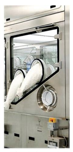
Figure 2: swissfillon's rapid transfer port used for ophthalmic fill  $\vartheta$  finish.
