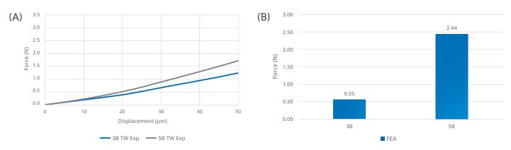
Figure 2: The finite element analysis confirmed a significantly lower hooked needle propensity for the five-bevel needle tip design compared with the three-bevel needle tip design. The trend (A) and external load (B) required to generate a hooked needle at 50 µm is significantly higher – approximately five times – for the five-bevel needle tip design than with the three-bevel needle tip design.
