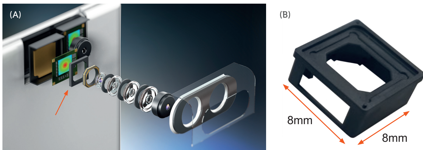
Figure 7: (A) Exploded view of compact camera (module frame identified by arrow). (B) Photograph of a compact camera module frame. Image courtesy adventrr / iStock / Getty Images Plus.
