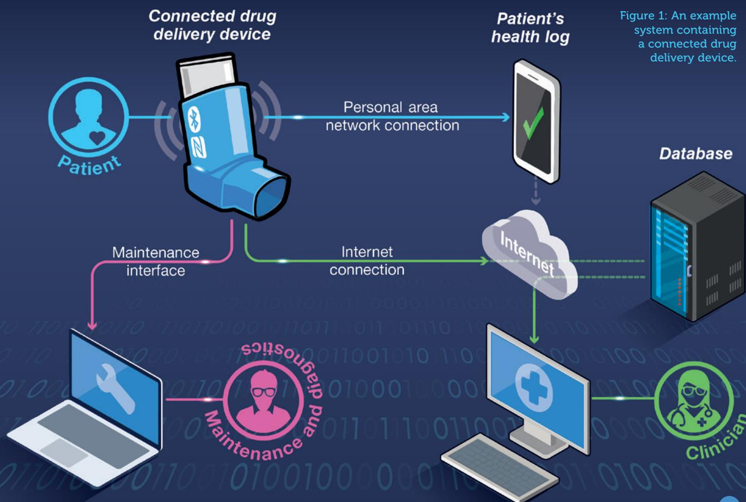
Figure 1: An example system containing a connected drug delivery device.
