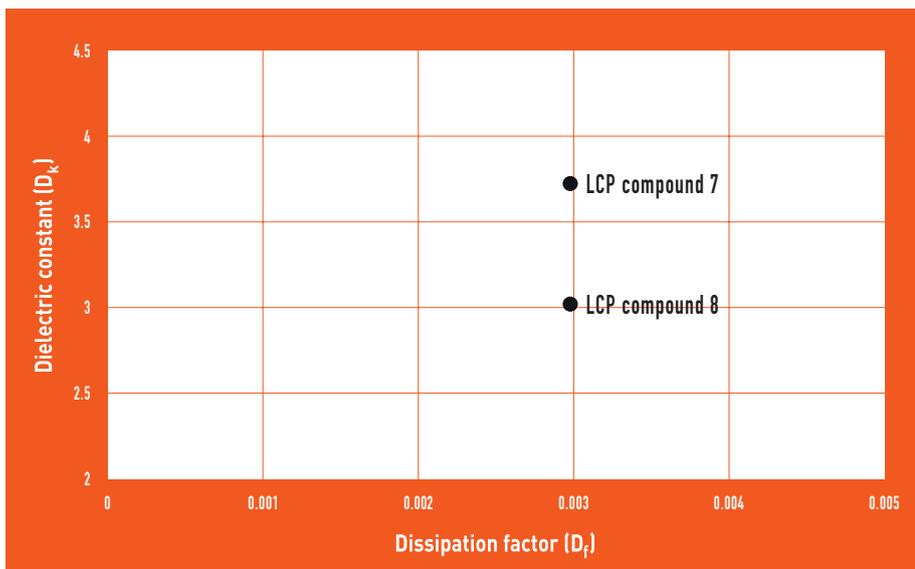
Figure 5:  $D_k/D_f$  values for low  $D_k$  Zenite LCPs, measured via IEC 61189-2-721 method at 2 GHz.
