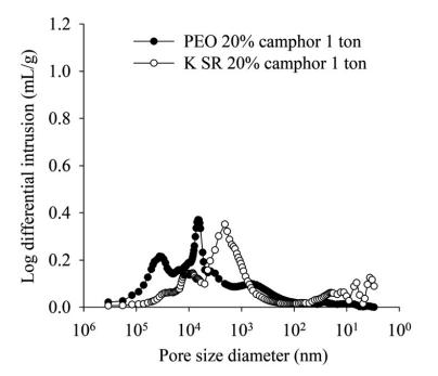
Figure 3: Fluid intrusion for two tablets with differing pore diameters.
