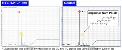
\* Quantification was achieved by integration of the GC-MS TIC signals and using a calibration curve of the external reference BHT.
