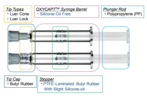
Figure 5: Components of an OXYCAPT™ syringe.
