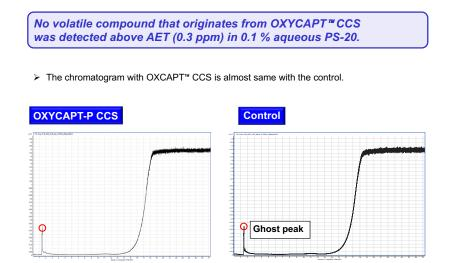
\* Quantification was achieved by integration of the HS-GC-MS TIC signals and using a calibration curve of the external toluene reference.
