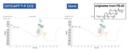
\* Quantification was achieved by integration of the LU-UV signals ( $\lambda$  = 220 nm) and using a calibration curve of the external reference BHT.
