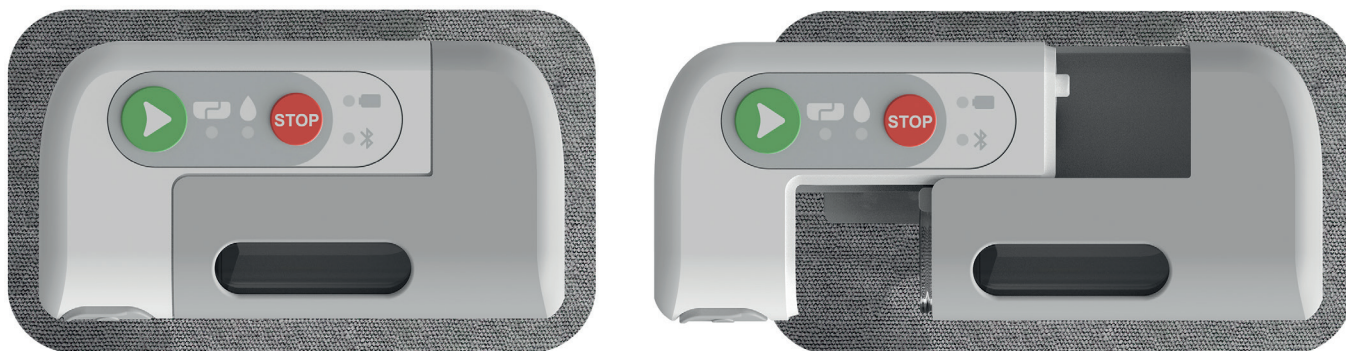
Figure 4: Symbioze consists of a reusable main unit and a prefilled, preloaded disposable module containing the drug.
