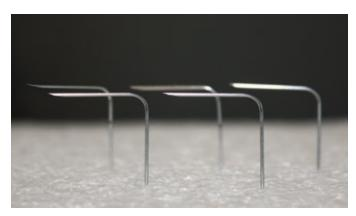
Figure 3: To ensure 100% safe use and functionality of the medical device, precise and repeatable needle bending needs to accommodate the input of imprecise bulk needles.
