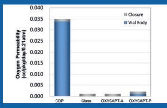
Figure 3: Oxygen permeability comparison of a typical COP, glass, OXYCAPT-A and OXYCAPT-P
