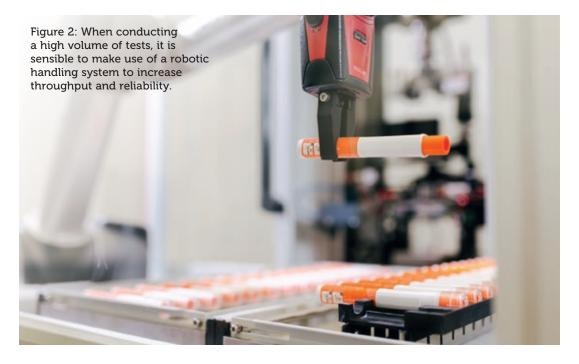
"With a high volume of tests, it makes sense to expand the testing machine with a robotic handling system. This ensures safe and economical testing of pharmaceutical packaging and medical products."
