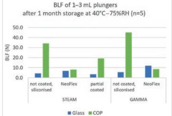
Figure 5: The above graphs show that uncoated and partially coated plungers give much higher break-loose forces then NeoFlex in COP barrels.
