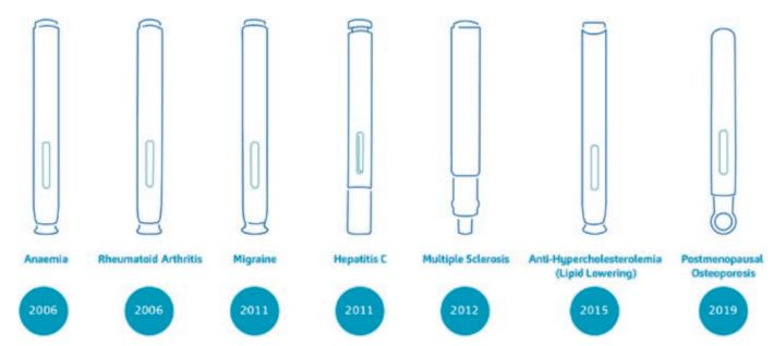
Figure 3. A non-exhaustive overview of combination products based on the DAI technology and their treatment areas. From the first DAI device, iterative developments over the years gave rise to devices inspired by the original version, and these were in the form of two- and three-step autoinjectors featuring manual or automatic needle insertion controls.
