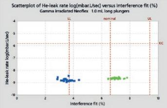
Figure 1: He-leak rates of gamma irradiated 1 mL long NeoFlex plungers with different interference fits. All cases easily meet the Kirsch Criterion (1.6x10–6 mbar.L/sec). Even with the worst-case scenario of a low interference fit, the seal integrity is still maintained.
