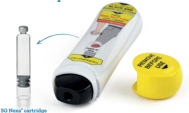
Maverick is an innovative emergency-use auto-injector designed for IM injection with integrated mechanical feature guaranteeing full dose delivery and automatic needle retraction mechanism. It is born by the collaboration between Stevanato Group and Duoject.
