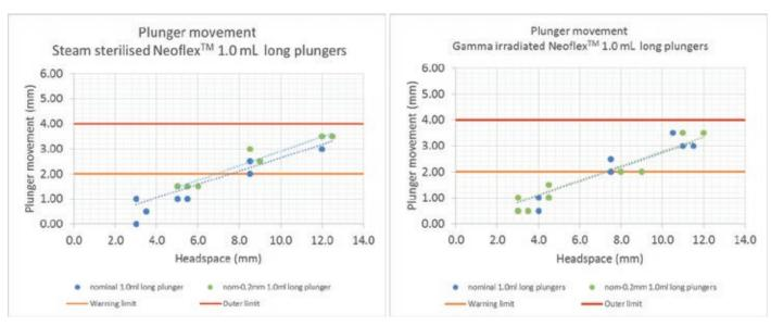
Figure 3: The above graphs show that, for plungers in a highly pressurised setting, plunger movement is minimal and well below the outer limit, regardless of whether the plungers were steam sterilised or gamma irradiated.
