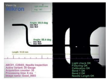
Figure 2: Mikron has become a leader in machine vision and the deployment of high-speed inspection systems to verify needle processing.
