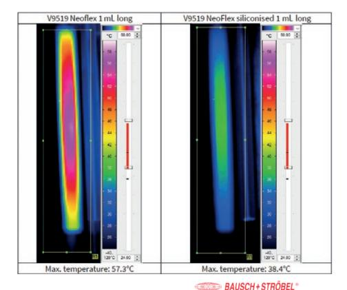
Figure 4: Temperature of vent tube in combination with NeoFlex 1 mL long and NeoFlex siliconised 1 mL long. Data provided by Bausch & Stroebel pharma services.
