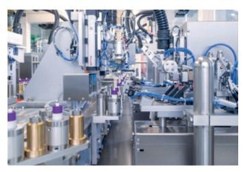
Figure 2: teamtechnik's high-speed assembly solution for pen injectors.
