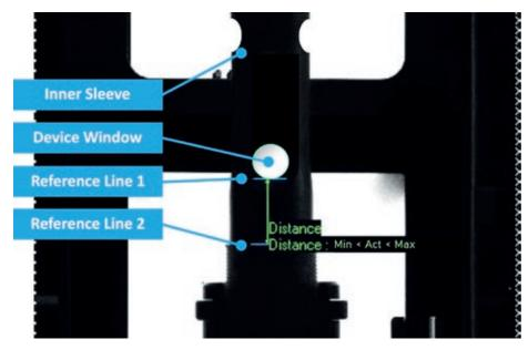
Figure 3: With 100% in-line controls, sensors can check, amongst other things, if device components are in the correct position, and if not, automatically reject the device.
