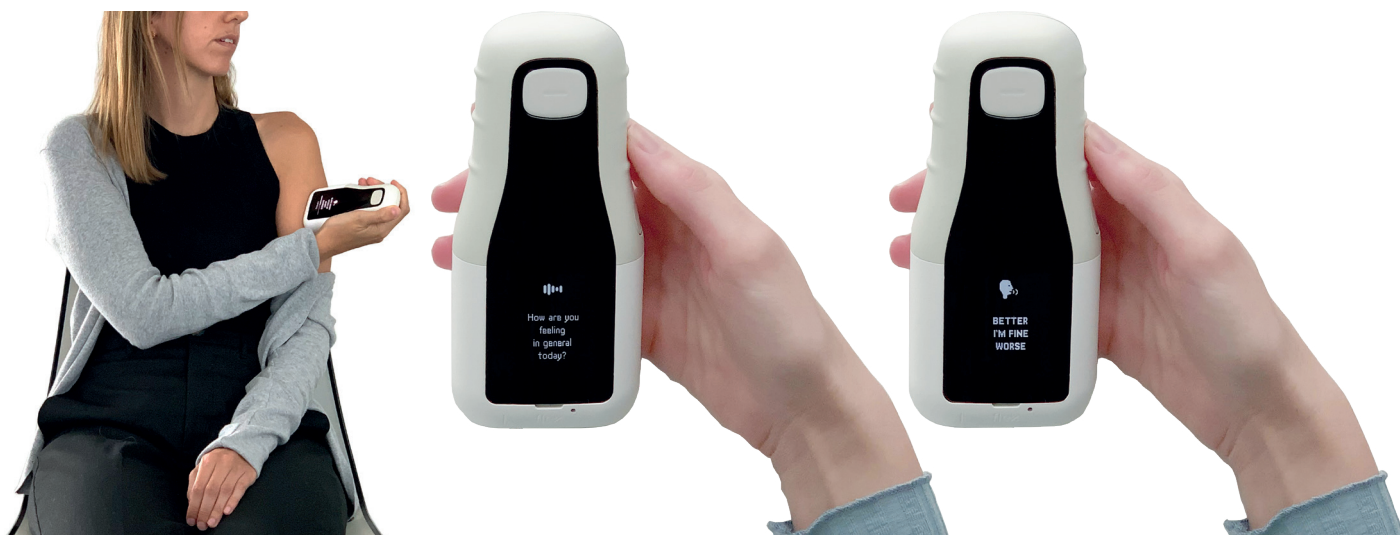
Figure 1: Autoinjector voice-interface. Assisted injection process and collection of patient feedback on health status.
