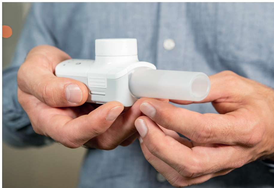
Figure 2: A handheld vibrating mesh device, which delivers nebulised drug products deep into the lungs.
