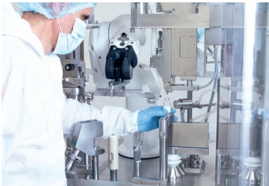
Figure 1: Close-up of 3P's Fill2Weight gravimetric filler in their R500 Robotic Capsule Filler.
