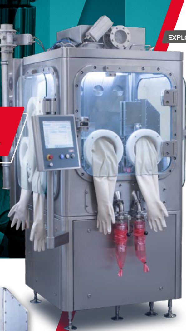
R500/R1000 Robotic powder dispensing for devices and capsules
