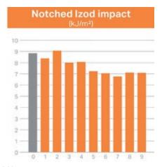
Figure 5: Physical properties of unsorted polycarbonate-based materials after multiple 100% regrind recycle loops.
