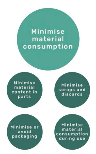
Figure 3: The four guidelines for the Ecodesign principle minimise material consumption.
