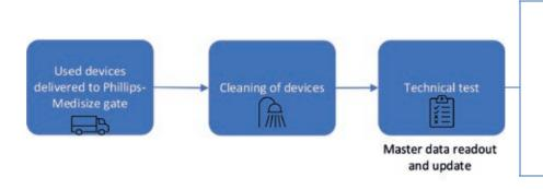
Figure 4: The refurbishment flow starts with devices being cleaned and tested. The device master data supplies information about the use cycle and can help determine if the device should be recycled due to high wear and tear or if there is a case for refurbishment, changing out worn parts like the plastic outer shell or the battery.
