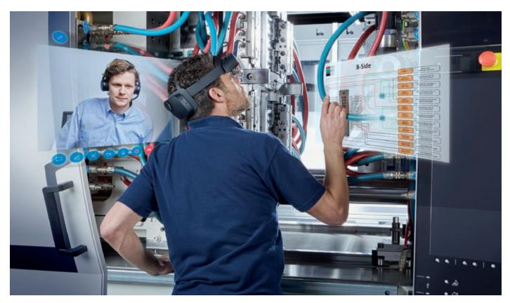
Figure 7: The HoloLens can project interactive holograms such as 3D-mould models, mould manuals and other files.
