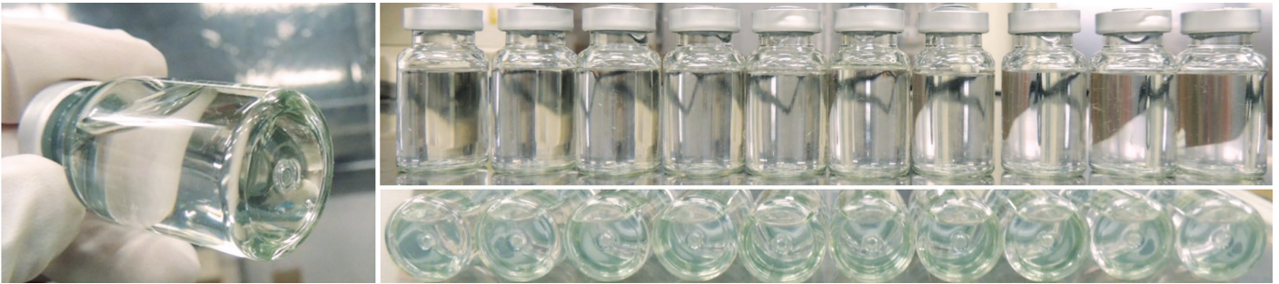
Figure 6: No breakage, leakage or layer separation was found after the quick defrosting test (-80°C to 40°C).
