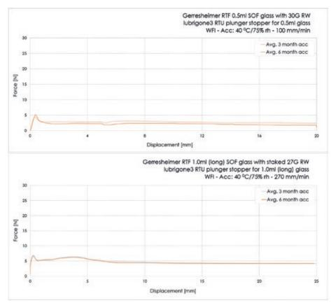
Figure 4: Examples of the break-loose and gliding-force profiles.
