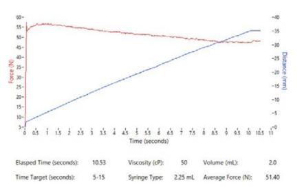
Figure 10: Altaviz test system graphical output showing position data and force profile.
