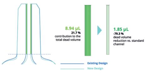
Figure 2: Dead volume reduction by optimising the internal cone design.
