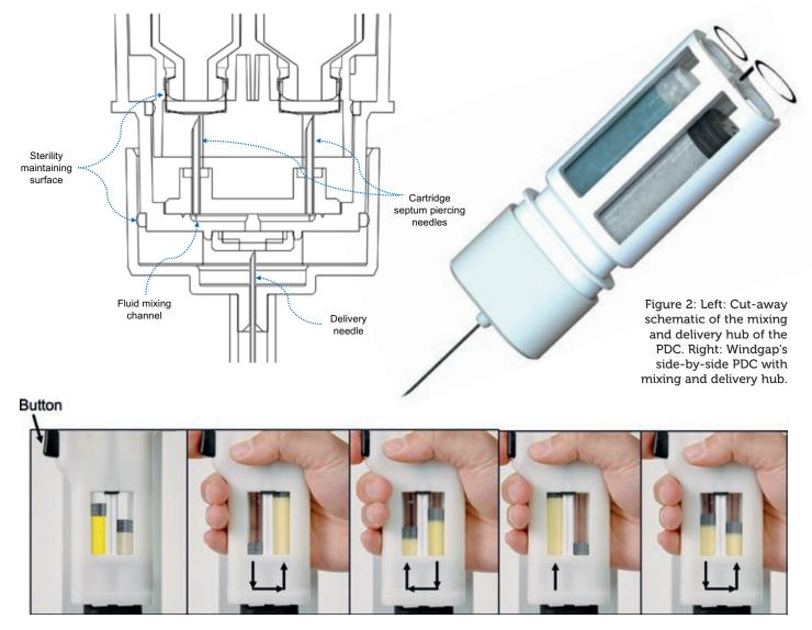
Figure 3: Demonstration of Windgap's reciprocating autoinjector mixing a cyanide antidote drug product currently under development. Arrows indicate alternating fluid flow in the PDC between cartridges.
