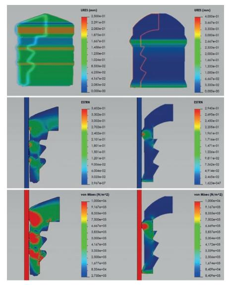
Figure 2: Simulating and comparing strain and stress profiles of unsiliconised lubrigone3 plungers and a coated butyl rubber plunger in glass, in the conversion from dynamic state to motion by combining a nonlinear simulation of hyperelastic using Mooney-Rivlin and a linear elastic deformation using Mohr-Coulomb. Left: Butyl rubber plunger stopper; Right: lubrigone<sub>3</sub> plunger stopper; Top: Deformation of plunger stopper; Mid: Maximum strain; Bottom: Maximum stress.
