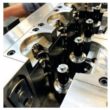
Figure 2: High-quality industrial line mould for glass-like safety devices.
