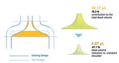
Figure 3: Dead volume reduction by optimising the internal shoulder design.
