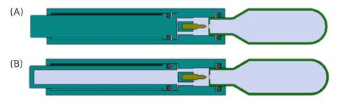
Figure 8: A more consistent force profile can be achieved by incorporating additional system volume (B) compared to a traditional layout (A).
