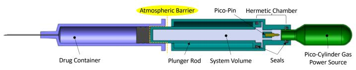
Figure 2: Gas pressure isolation from primary drug container.
