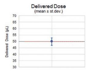
Figure 5: The extruded doses closely aligned to the 50  $\mu L$  target dose.
