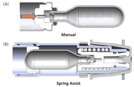
Figure 9: Two Pico-Cylinder deployment concepts.
