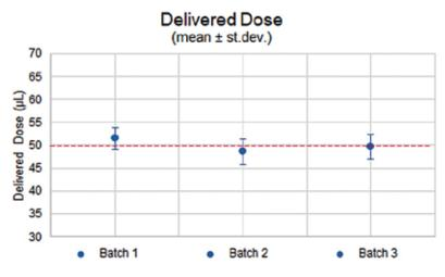
Figure 4: High degree of consistency of the delivered dose across three batches.
