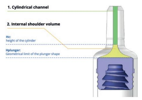
Figure 1: The cone and the shoulder design is a key element to reaching dose accuracy.
