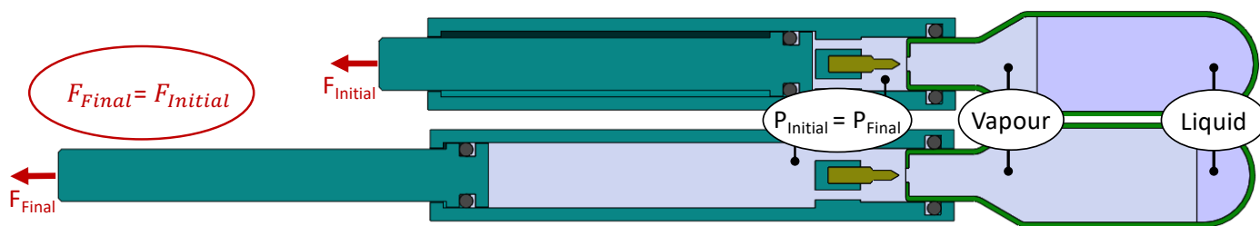
Figure 5: Dual-phase gases provide a constant pressure at a set temperature resulting in a constant force profile.
