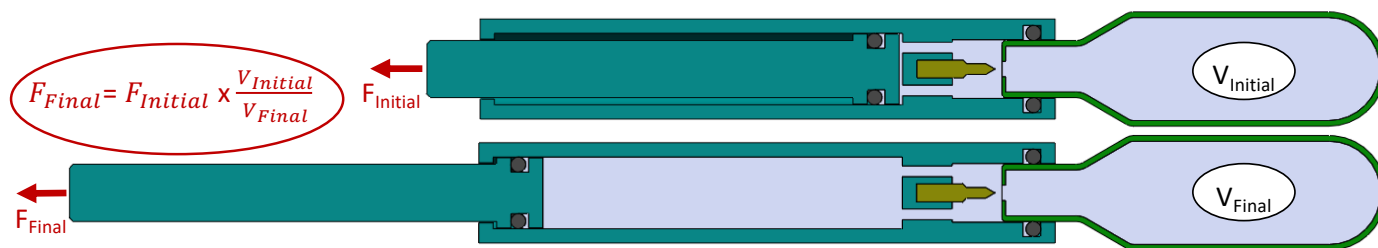
Figure 6: Force drop over stroke due to increase in internal volume as plunger deploys.
