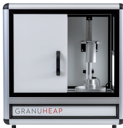
Figure 4: GranuHeap – an automated AOR measurement device.
