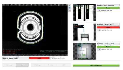
Figure 1: Inspection module with a variety of device verification checks.
