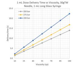
Figure 4: Small needle gauge delivery model data.
