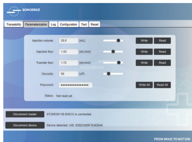
Figure 4: Near-field communication interface for parameterisation of the device’s volume and flow rate depending on drug viscosity.
