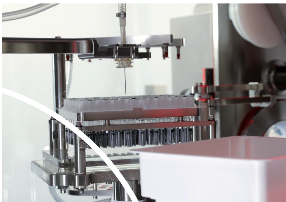
Figure 1: Aseptic syringe filling using advanced robotic isolator technology.
