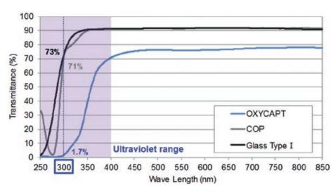
Figure 4: UV light transmittance comparison of a typical COP, Type 1 glass and OXYCAPT.
