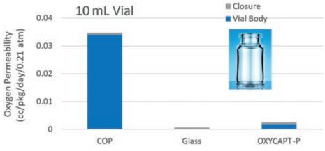
Figure 3: Oxygen permeability comparison of a typical COP, glass and OXYCAPT-P.
