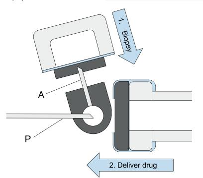
Figure 2: Schematic illustrating VitreoDx's unique fluidic system for acquiring a neat biopsy of vitreous fluid prior to injecting the drug. Arrows indicate the lateral pressing motion of the button to impale the evacuated biopsy chamber on the accessory needle (A), followed by the axial sliding motion of the button to impale the drug cartridge on the primary needle (P).
