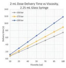
Figure 2: Dose delivery time versus viscosity model data.
