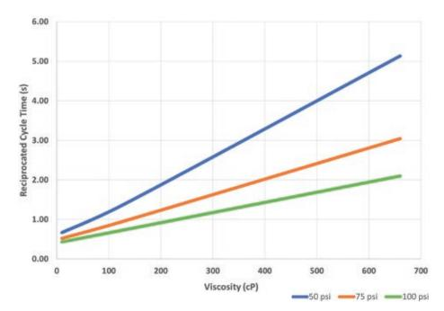
Figure 2: The time in seconds to complete one mixing cycle for a 3 mL dose is shown with respect to applied pressure for a range of viscosities. Data include the time required to actuate valving and pressurise the system at the beginning of each test.
