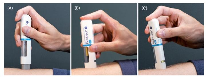
Figure 2: (A) PiccoJect directly before injection with the cap already removed. (B) PiccoJect during injection – the yellow plunger moves down in the large wrap-around drug window. (C) PiccoJect immediately after the injection is finished – the status indicator shows that injection is completed.
