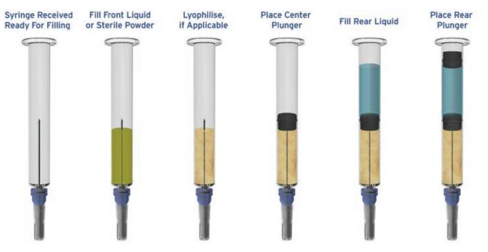
Figure 2: The fill-finish process for a prefilled dual chamber syringe.
