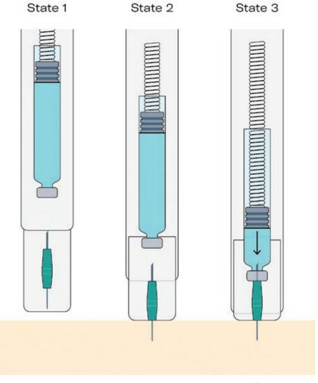
Figure 2: An overview of the injection mechanism of the Gx Inbeneo<sup>®</sup>, showing how the fluid path is established in a single user step.
