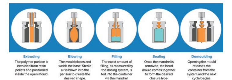
Figure 5: BFS technology creates, fills, seals, inspects and labels a container in a single integrated process that takes 3-7 seconds.
