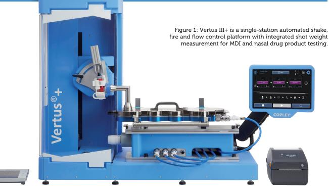
applies the same rotational shaking motion to appropriately represent patient/analyst practice and, at the same time, enable straightforward method transfer. Each benefits from electronic records/electronic signatures (ERES) functionality, providing a basis for obtaining ERES regulatory approval compliant with 21 CFR Part 11 requirements.
