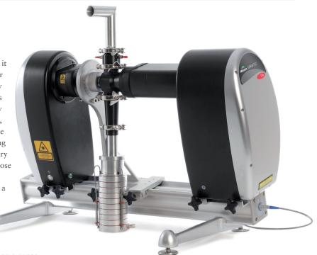
Figure 3: Spraytec laser diffraction system with inhalation cell.
