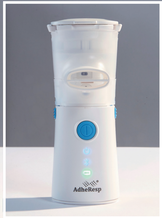
Figure 1: AdheResp – a smart, breath-actuated mesh nebuliser.
