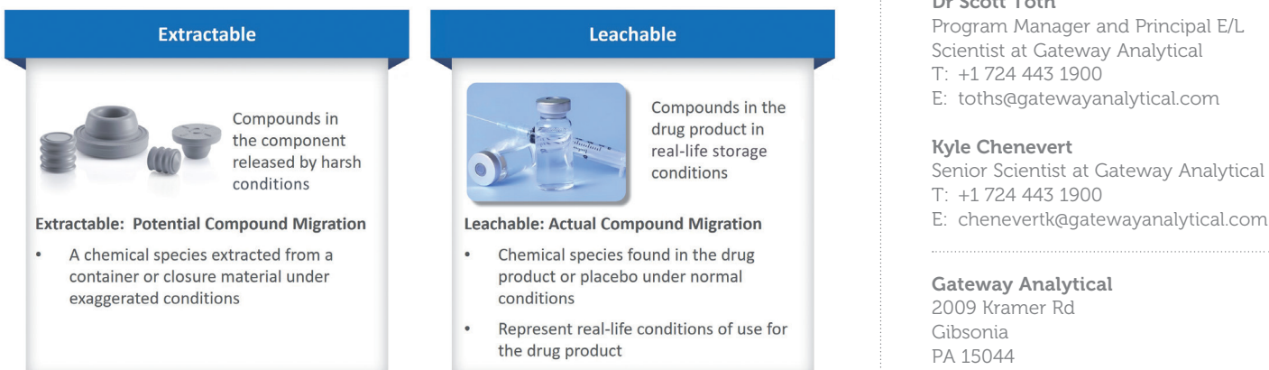
Figure 1: Extractables are compounds that could migrate into the product; leachables are compounds that migrate into the product under representative conditions.
