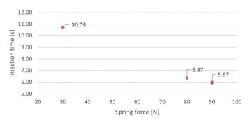
Figure 4: Injection times of 3 mL of 1 cP liquid (water) at three different force levels using the Gx Inbeneo® platform simulator.
