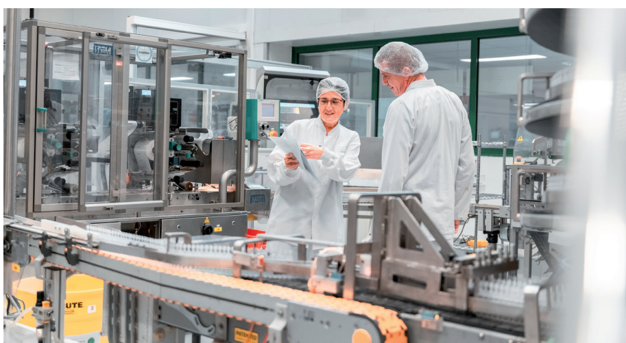
Figure 3: Fully automated BFS production at Unither's Amiens facility.
