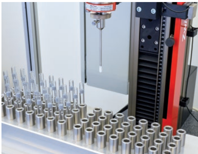
Figure 1: Sequential testing systems save time and significantly reduce operator influence.
