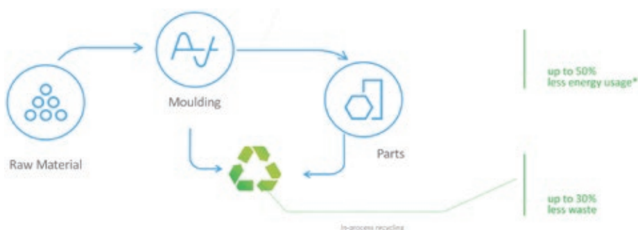
Figure 3: The process for producing thermoplastic elastomers, leading to major reductions in energy usage and waste production compared with that for thermoset rubbers (*calculations based on non-medical commercial part).
