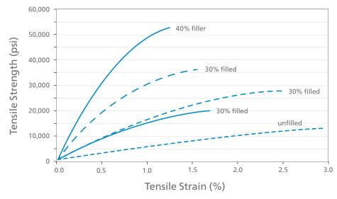
Figure 2: PEEK is a versatile base polymer that can be customised with suitable fillers to impart different properties.
