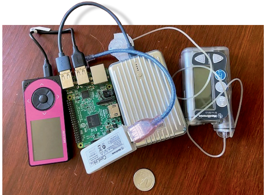
Figure 4: A DIY artificial pancreas system from 2016, using a battery-powered Raspberry Pi, Dexcom receiver, and CareLink USB stick transmitting to a Medtronic pump. 16
