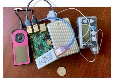
Figure 4: A DIY artificial pancreas system from 2016, using a battery-powered Raspberry Pi, Dexcom receiver, and CareLink USB stick transmitting to a Medtronic pump.<sup>16</sup>
