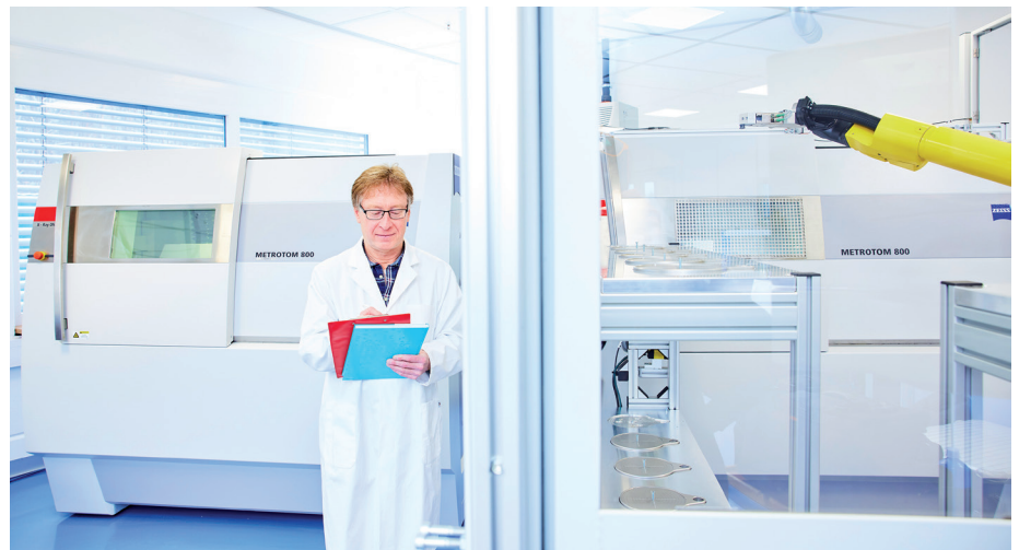
Figure 7: Industrial CT scanner for the destruction-free measuring and testing of individual components or entire assemblies.
