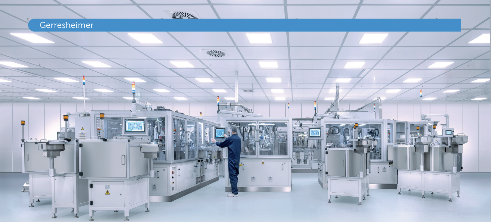
Figure 3: High-volume drug delivery device assembly room in an ISO Class 8 cleanroom in Pfreimd (Germany).
