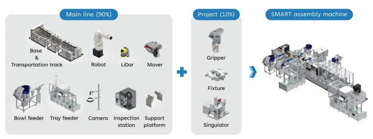
Figure 1: Non-exhaustive key reusable and project-specific modules of a SMART assembly machine.
