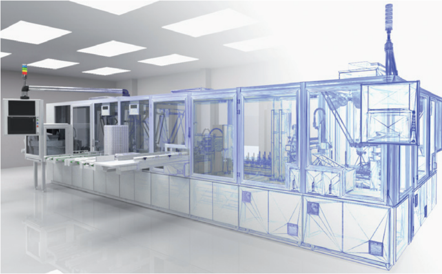
Figure 2: Stevanato Group’s digital twin is a digital replica of a physical entity. Applied to assembly equipment, it allows process optimisation in the design phase.
