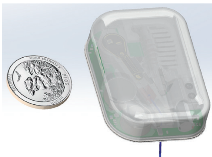
Figure 4: The Horizon I all-in-one wearable injector.
