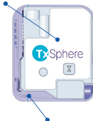
DDC module (disposable drug container) with integrated cannula injector
