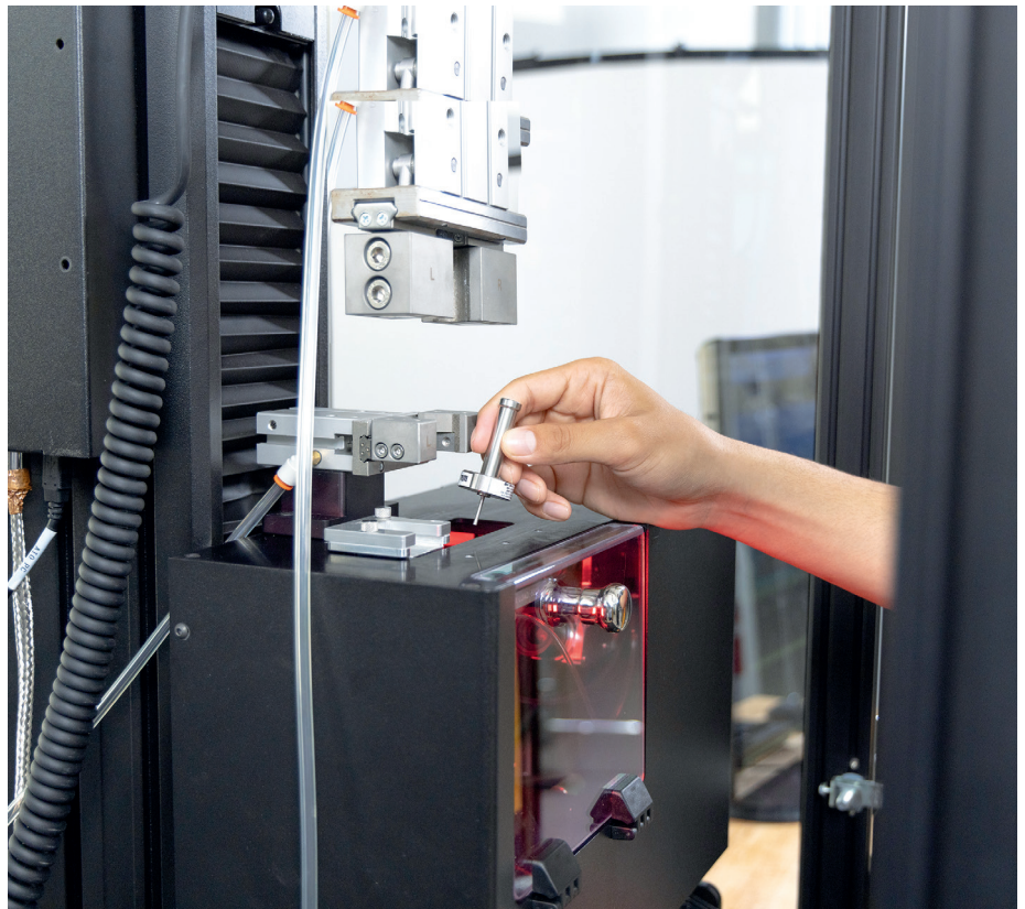
Figure 5: Operator uses gauge pins to verify camera performance for system suitability testing.
