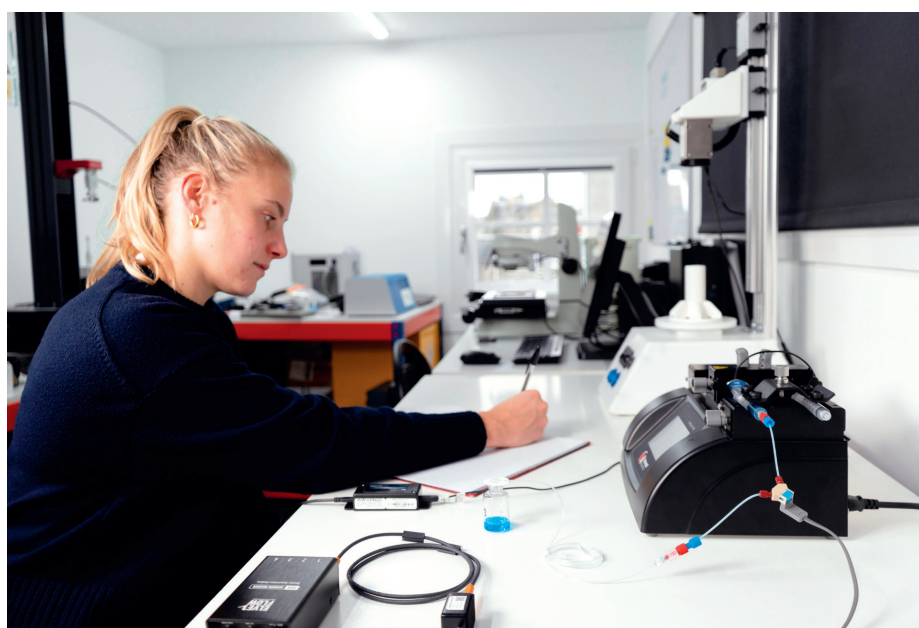
Figure 5: Equipment such as a universal test machine or syringe pump can simulate a drive system.
