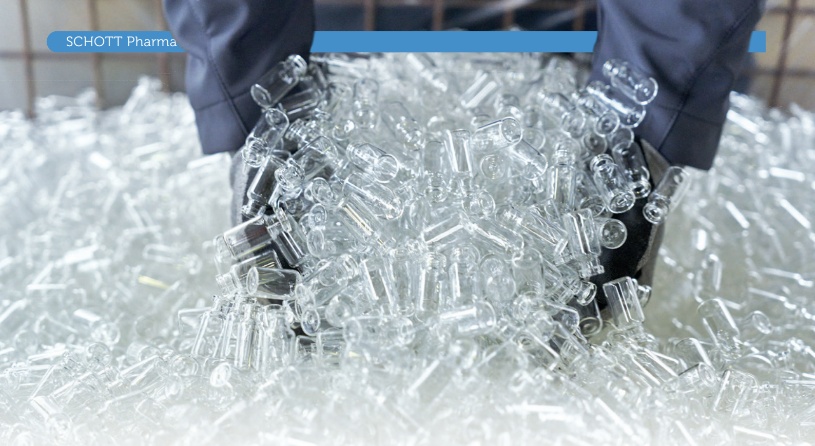
Figure 3: Glass vials for turning back into high-quality pharmaceutical glass tubing.
