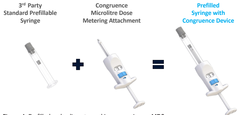
Figure 4: Prefilled embodiment – making any syringe a MDS.
