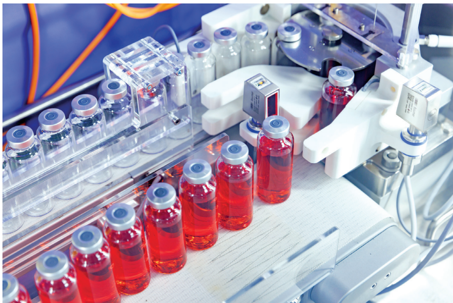
Figure 1: InnoMedica's innovative closed-vial filling system for clinical and early-market scale production.
