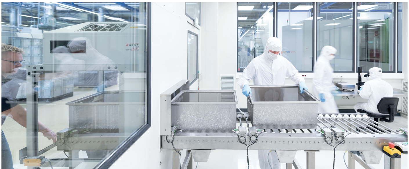
Figure 2: STÜKEN MEDICAL operates Class 7 cleanrooms in accordance with DIN EN ISO 14644 and EU GMP Class C guidelines.
