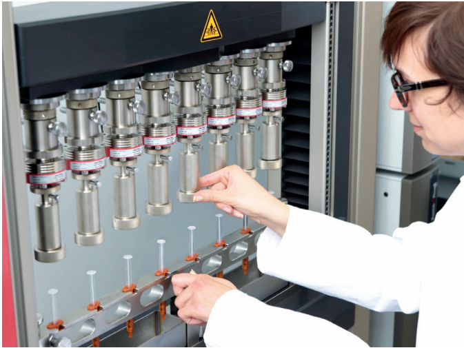
Figure 4: Eight syringes tested simultaneously, with individual test results and values recorded separately.
