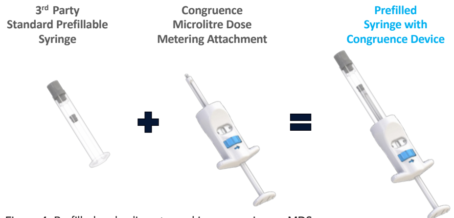
Figure 4: Prefilled embodiment – making any syringe a MDS.
