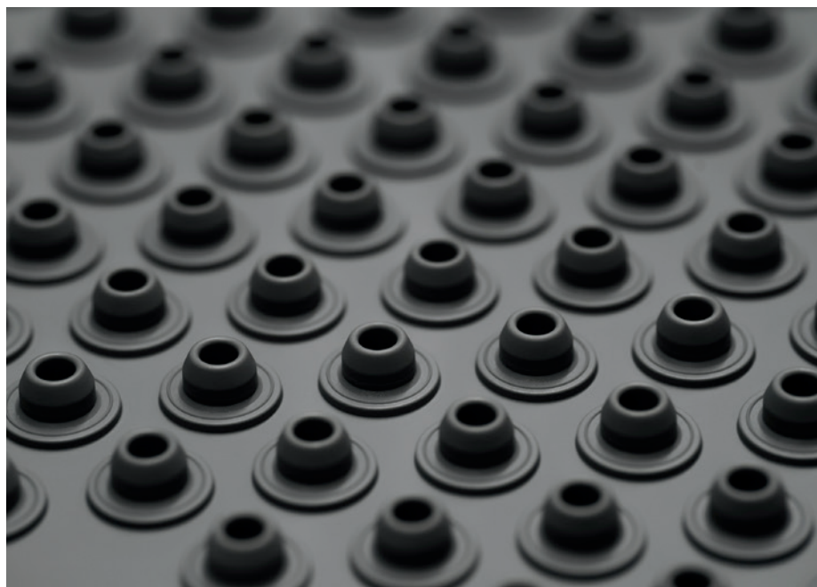
Figure 1: Aptar Pharma vial stopper sheet. Downstream vulcanised rubber scraps enter a recycling network.
