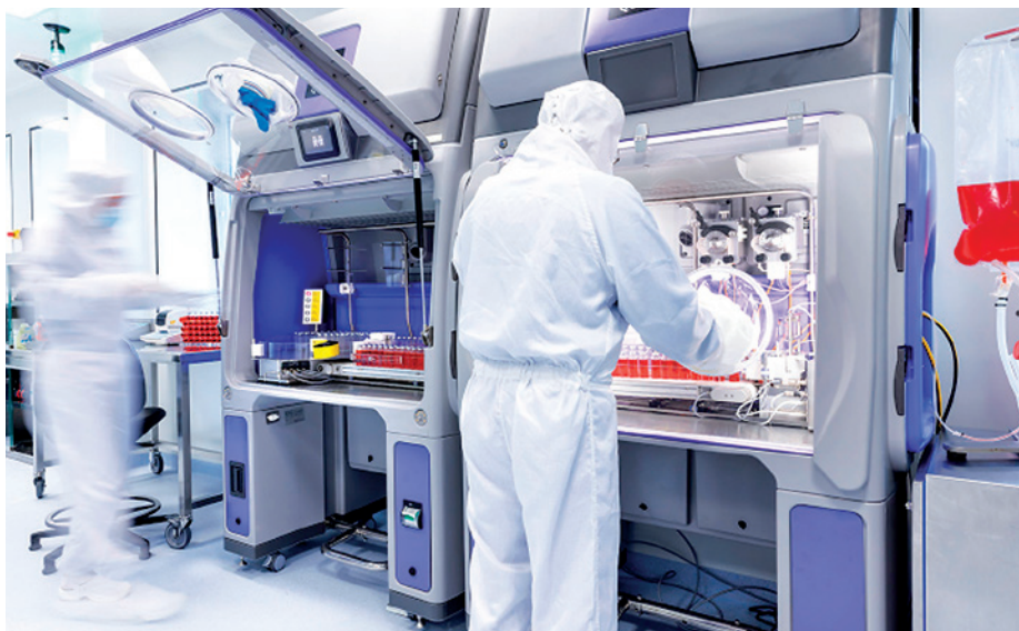
Figure 2: The closed vial filling system can pierce a vial's septum without compromising container integrity.
